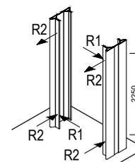
LE SPINTE R1 E R2 POSSONO ESSERE APPLICATE A QUALSIASI PUNTO DELL'ALTEZZA DEL VANO CORSA
