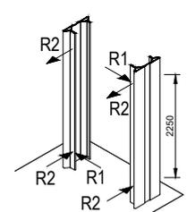
LE SPINTE R1 E R2 POSSONO ESSERE APPLICATE A QUALSIASI PUNTO DELL'ALTEZZA DEL VANO CORSA
